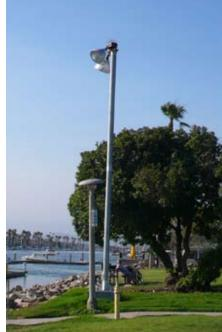
below 0.001 footcandles), to unecessarily high levels of illumination (pools of light from spotlights exceed 50 footcandles). Ideally, the illumination along the pathway would range from 0.25 to 10 footcandles (see Table 1 for summary of recommended illuminance guidelines), with an average of 1 footcandle.
