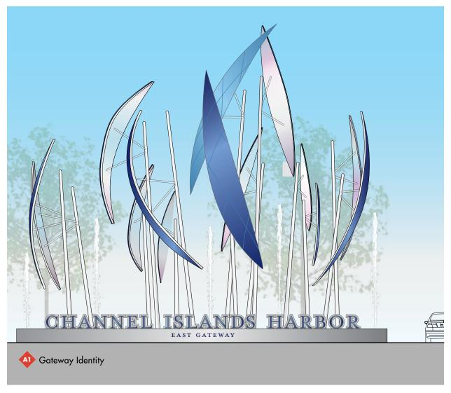
halo illumination with remote transformers. "WEST GATEWAY" letters to be flat cut-out painted ½" thick aluminum letters pin mounted to concrete, or 1" deep letters cast into concrete (debossed).
